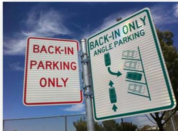
Figure 21 Sample Back-In Angle Parking Signs
