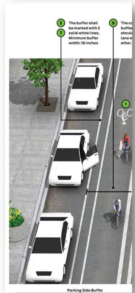
Figure 9 Example of Pavement Markings for Door Zone
